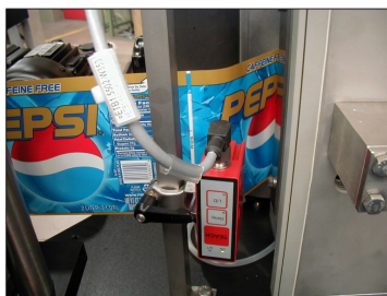
Fig. 73: Sensory scanning of a register mark
