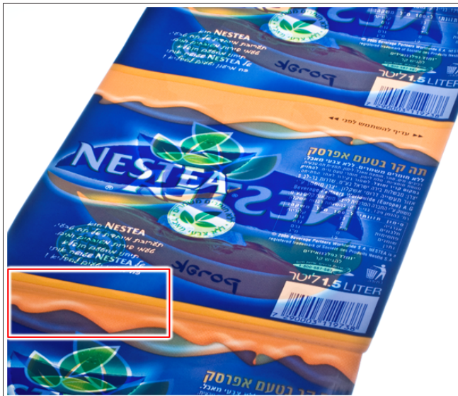
Fig. 116: Readable luminescent register mark
