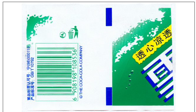
Fig. 95: More than one colour in the scanning area before and after the register mark
