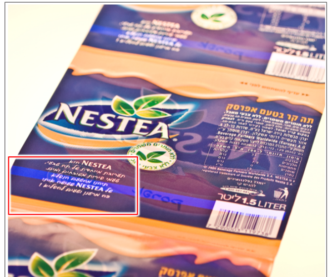
Fig. 117: Readable luminescent register mark
