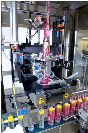
Fig. 114: Example of sensory scanning of a register mark
