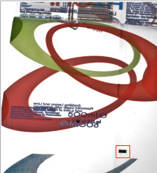
Fig. 120: Readable colour contrast register mark
