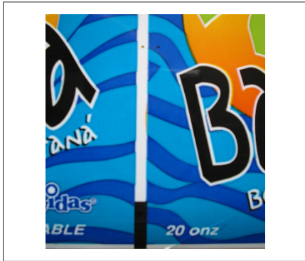
Fig. 91: More than one colour in the scanning area before and after the register mark and colour contrast not sufficient
