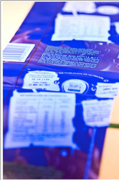
Fig. 119: NON-readable luminescent register mark
